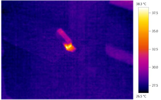
Thermal Image of Mild steel Sample after 2 secs of failure
