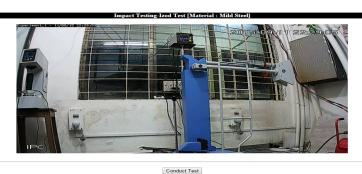
Status: Receiving.... Energy Absorbed during Impact Test = 26 Joules
